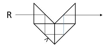
a) Draw the tunnel diagram and indicate the orientation and parity of the letter "R" as viewed through the prism system.
