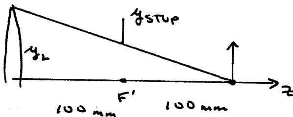
The chief ray height at the lens must equal the object size by telecentricity.  $y_L = 10$
