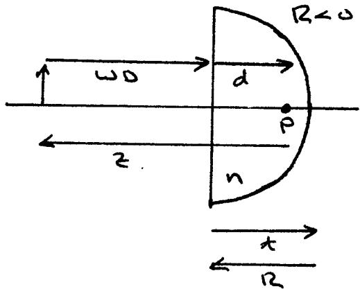
From imaging:  $f = 3.4 \text{ mm}$        $z = -3.47 \text{ mm}$
