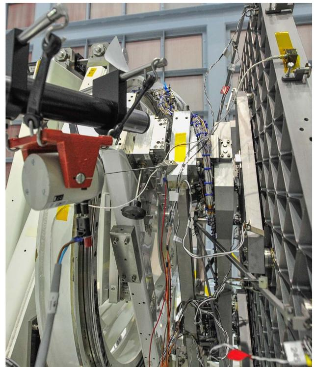
**Fig. 3.** This photograph shows how the stinger was positioned and connected to the mirror support structure (the back side of the mirror is visible on the extreme right and has a triangular rib structure). The stinger is the cylindrical object mounted in the red bracket on the extreme left. There is a force sensor interposed between the stinger rod and the structure.
