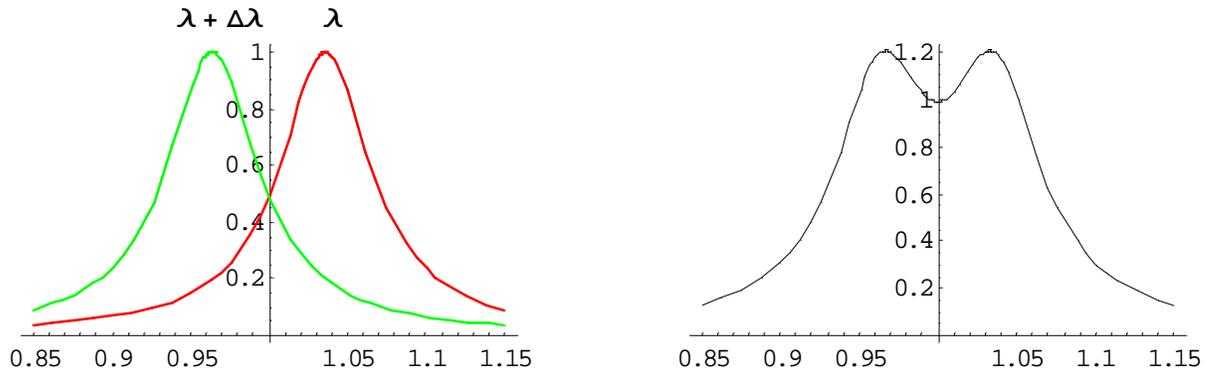
The left side of the figure shows the individual intensity contours of two Fabry-Perot fringes that are just resolved. The right side shows the two intensity contours added to give the observed effect.
