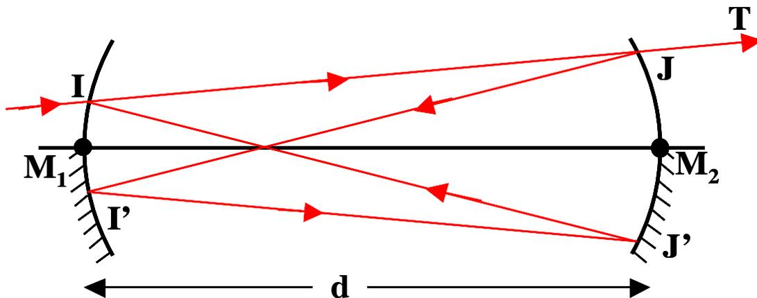
In the paraxial region the path difference between the initial ray  $IJ$  and ray  $IJJ'IJIJ$  is equal to  $4d$ , where  $d$  is the distance between  $M_1$  and  $M_2$ .
