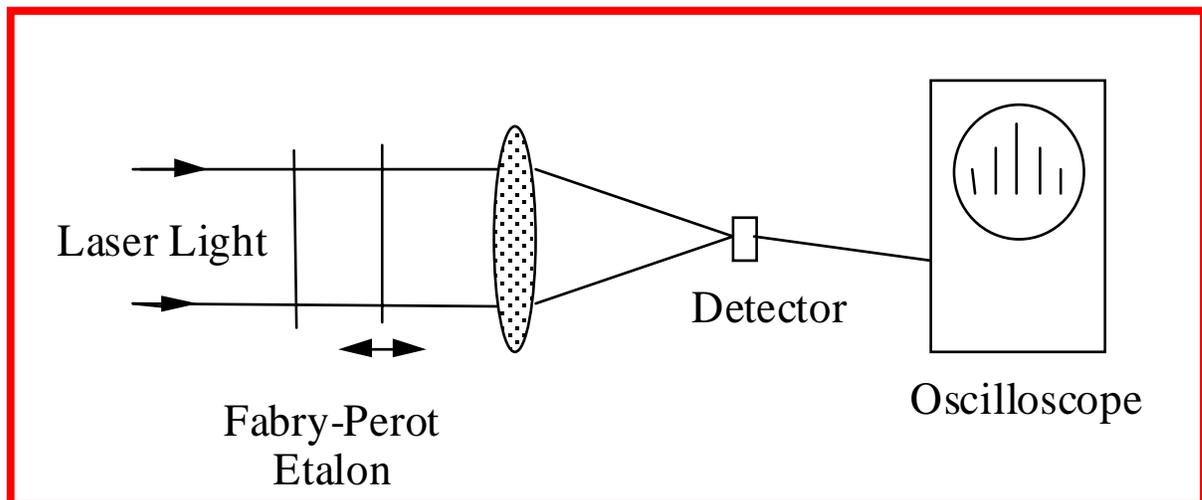
The scanning can be achieved by mounting one of the Fabry-Perot mirrors on a PZT. Since for a given fringe
