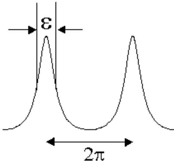
$$\text{finesse} = \frac{\text{separation of adjacent fringes}}{\text{width of half max}}$$
