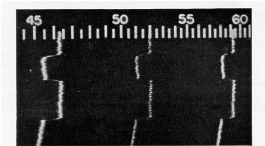
Fig. 7.79. Fringes of equal chromatic order given by a section of a diamond crystal surface. The scale is of wavelength in hundreds of Ångstroms. (After S. TOLANSKY and W. L. WILCOCK, *Proc. Roy. Soc., A*, **191** (1947), 192.)
