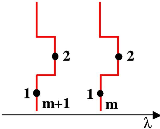
$$d = \left(m - \frac{\phi}{\pi}\right) \frac{\lambda}{2} \quad \text{and} \quad d_2 - d_1 = \left(m - \frac{\phi}{\pi}\right) \left(\frac{\lambda_{2,m} - \lambda_{1,m}}{2}\right)$$
