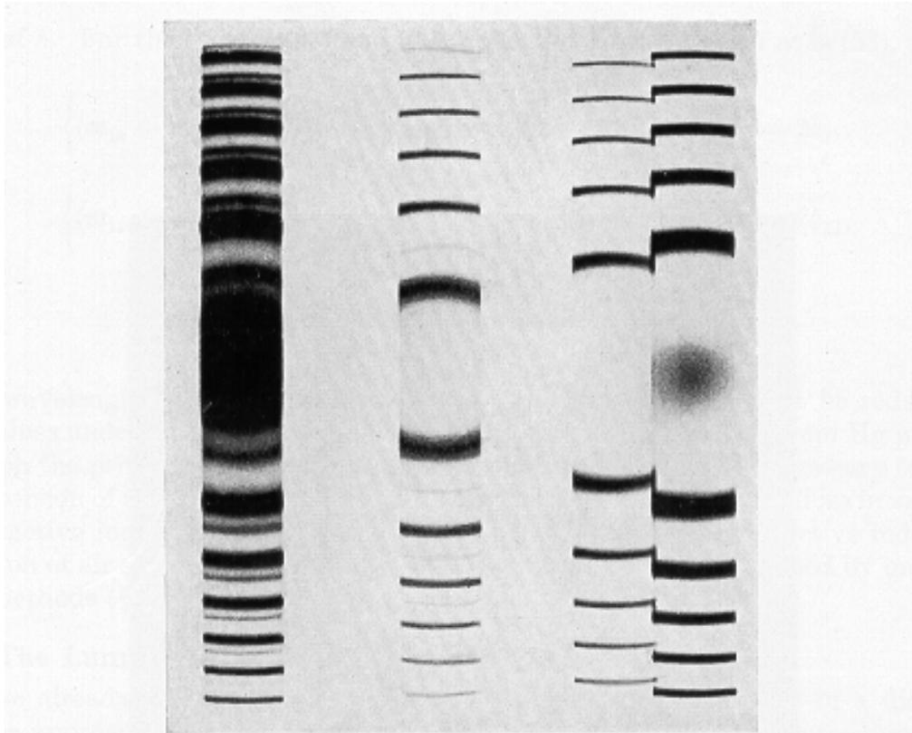
Fig. 7.64. FABRY-PEROT fringes from lines in the emission spectrum of helium (photographic negative).
