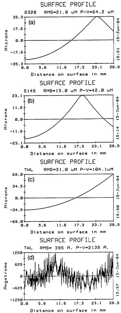
Fig. 5. (a) Single-wavelength data obtained at  $\lambda = 6328 \text{\AA}$  showing breakdown of phase measurement when the wave front slope is too steep. (b) Similar data as in (a) but  $\lambda$  is changed to 5145  $\text{\AA}$ . (c) The equivalent wavelength ( $\lambda_{eq} = 2.75 \mu\text{m}$ ) data. (d) Same data as in (c) but with both tilt and focus removed.
