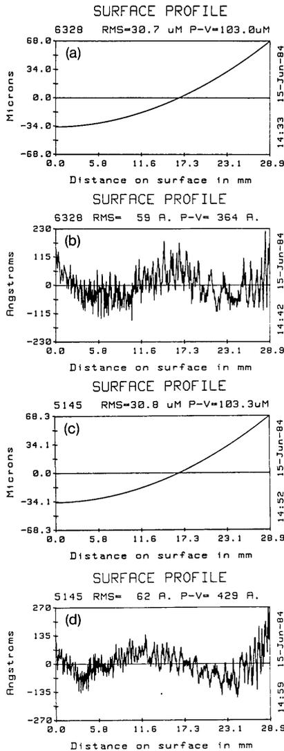
Fig. 6. (a) Single-wavelength data obtained at  $\lambda = 6328 \text{ \AA}$  with  $2\pi$  ambiguities corrected. (b) Same data as in (a) but with both tilt and focus removed. In (c) and (d) the wavelength was changed to  $5145 \text{ \AA}$ .
