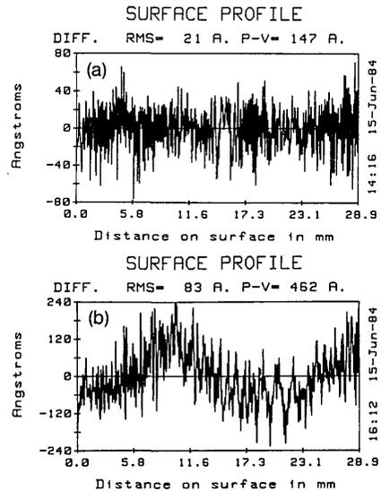
Fig. 7. (a) Repeatability of the surface height measurement without temporal averaging by the second method of TWLPSI (obtained at  $\lambda = 6328 \text{ \AA}$ ). (b) Difference between the data sets in Fig. 6(b) ( $\lambda = 6328 \text{ \AA}$ ) and Fig. 6(d) ( $\lambda = 5145 \text{ \AA}$ ).
