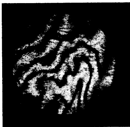
Fig. 7. Double exposure holographic interferogram of forced turbulence present in interferometer ( \lambda = 0.5145 \mu ).
