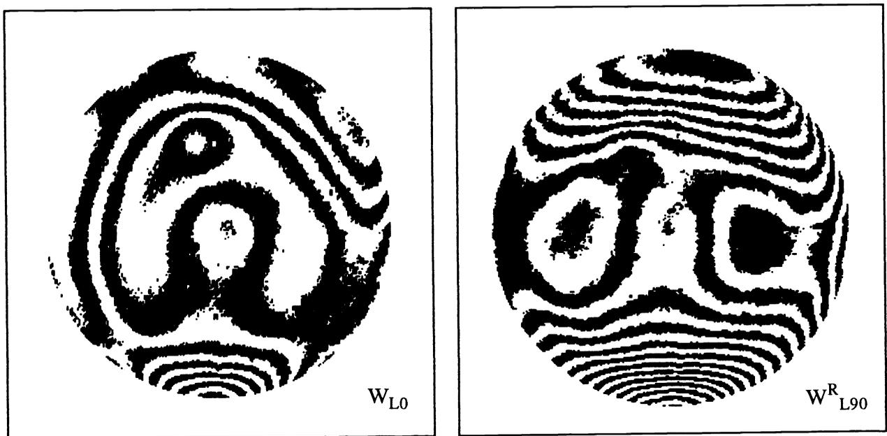
Fig. 5. The two measurement results, obtained with light linearly polarized in the vertical, in which the rod was oriented at  $0^\circ$  and  $90^\circ$ , respectively.  $W_{L90}^R$  is mathematically rotated back to the orientation  $0^\circ$ . This difference between them shows that the astigmatism is different for the two polarization states.
