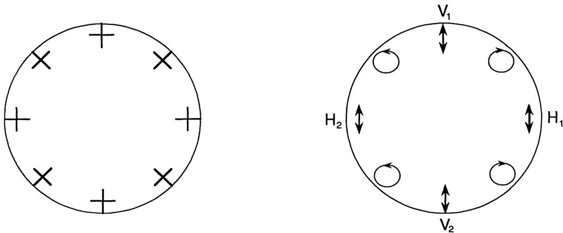
Fig. 2. (A) The principal directions of the stress in the cross section of the rod. They are either parallel or orthogonal to the radius. (B) For incident light linearly polarized in the vertical, the polarization remains unchanged in four orientations,  $V_1$ ,  $V_2$ ,  $H_1$ , and  $H_2$ .
