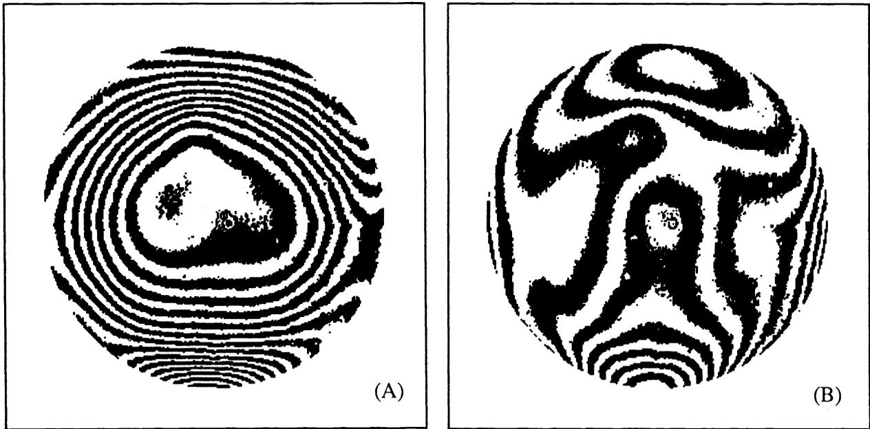
Fig. 4. (A) The measurement result obtained with circularly polarized light,  $W_{C0}$ , in which the rod was oriented at  $0^\circ$ . There is a strong defocus contribution. (B) The same result with the defocus contribution removed. All  $W_{C0}$ ,  $W_{C90}$ ,  $W_{C180}$ , and  $W_{C270}$  are very similar and have the same defocus contributions. This shows the rod has a rotational symmetry in birefringence. The interval of the isometric contour in Figs. 4 and 5 is 0.05 waves.
