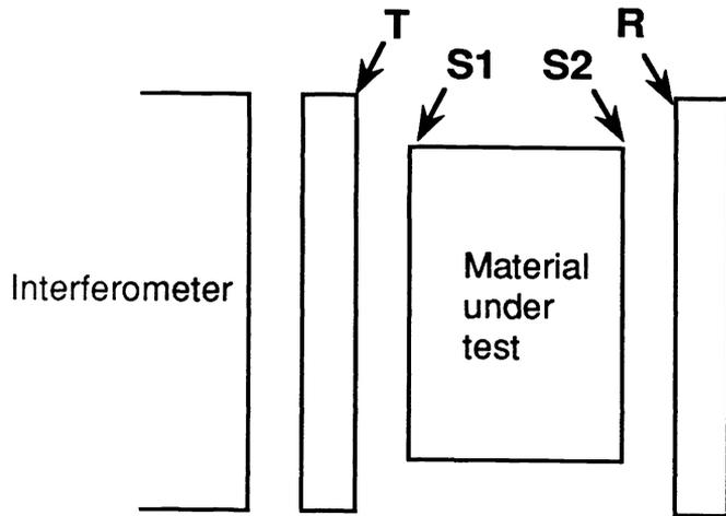
Fig. 1. The schematic diagram of the experimental setup. T is the transmission flat and R is the return flat.
