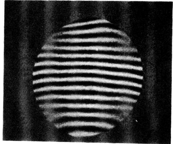
Fig. 3. The interference fringes have low contrast at the four 45 degree corners, obtained with a collimated beam linearly polarized in the vertical direction.
