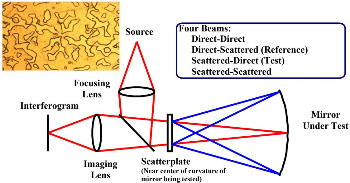
Figure 1. Scatterplate Interferometer for Testing Concave Mirrors.
