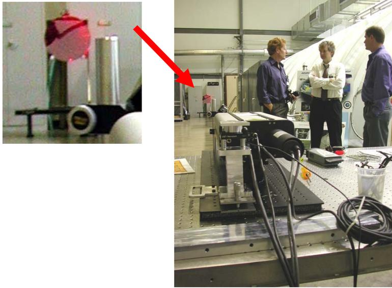
Figure 9. Use of PhaseCam to test a 0.5 meter diameter, 20 meter ROC mirror without any vibration isolation.
