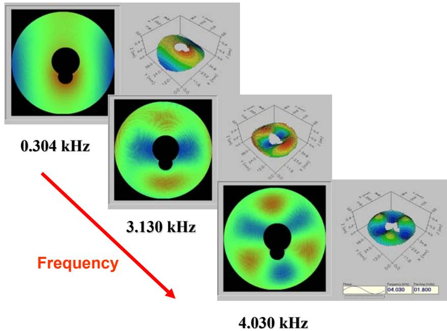
Figure 10. Vibrational modes of a disk.
