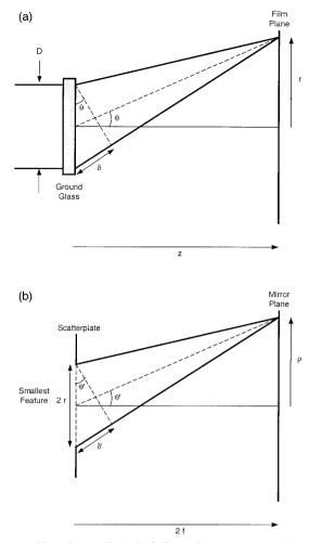
Fig. 12. f/number analysis for holographic exposure: (a) recording geometry, (b) interferometer geometry.
