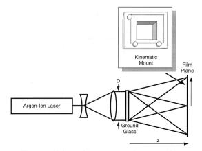
Fig. 11. Holographic exposure of a scatterplate.
