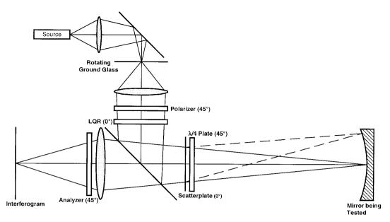
Fig. 6. Phase-shifting scatterplate interferometer. LQR, liquid-crystal retarder.
