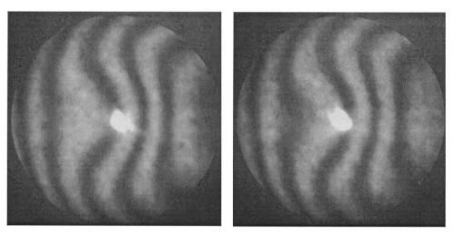
Frame 3 Frame 4 Fig. 7. Phase-shifted fringe patterns.
