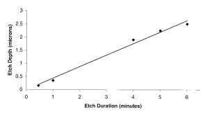
Fig. 9. Etch depth versus etch time for calcite in diluted HCl.
