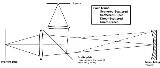
Fig. 1. Scatterplate interferometer for the testing of concave mirrors.
