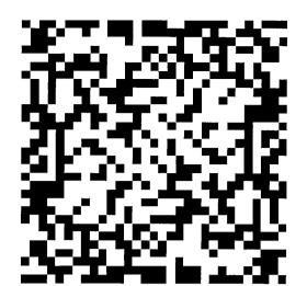
Fig. 2. Inversion symmetry designed into a binary scatterplate.
