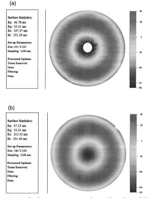
Fig. 13. (a) Surface measurement taken with a phase-shifting scatterplate interferometer. (b) Surface measurement taken with a Wyko 6000 phase-shifting Fizeau interferometer.
