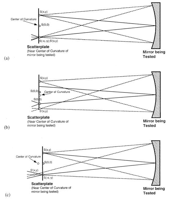
Fig. 3. Point-to-point analysis of inversion symmetry: (a) perfect alignment, (b) lateral misalignment of scatterplate, (c) longitudinal misalignment of scatterplate.
