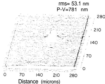
Fig. 8 Surface plot of high asperity present on Tape A
