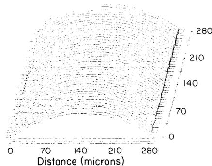
Fig. 9 Surface plot of a magnetic head with a cylindrical contour radius of 20 mm
