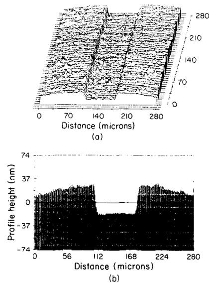
Fig. 3 Plots of a calibration standard. (a) Surface plot. (b) Profile in the x axis.
