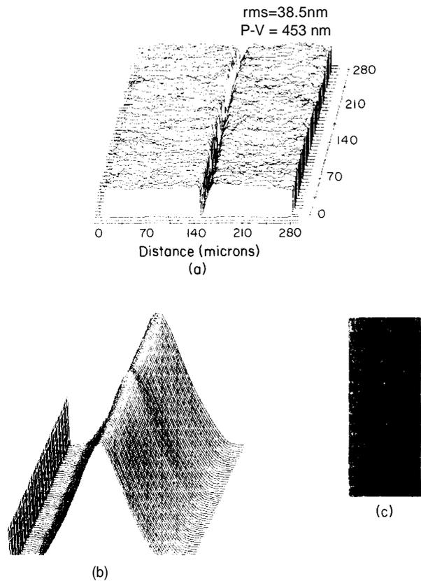
Fig. 7 Example of wear scratch on the tape surface (the longitudinal direction of the tape is along the vertical direction). (a) Surface plot. (b) Autocovariance function. (c) Contour for which autocovariance is greater than 0.1.
