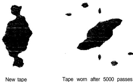
Fig. 6 Plot showing the points for which the autocovariance is greater than 0.1. The longitudinal direction of the tape is along the horizontal direction.
