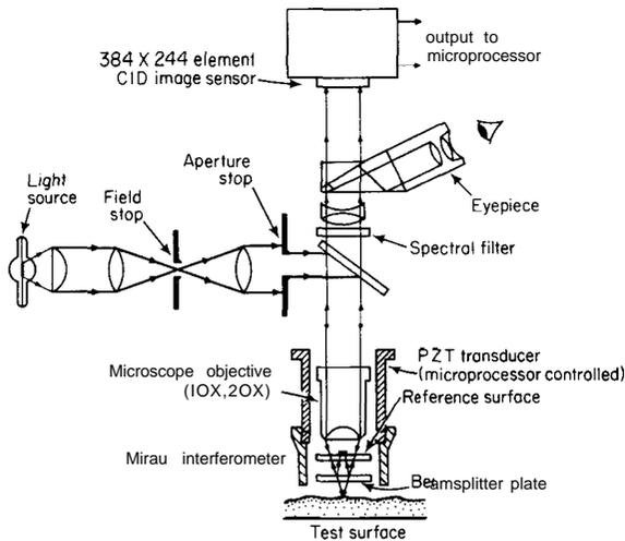
Fig. 1 Schematic of the three-dimensional digital optical profiler
