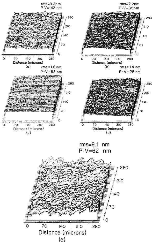
Fig. 5 Surface plots. (a) Rigid disk, radial direction along horizontal axis. (b) Lapped Ni-Zn ferrite. (c) Silicon wafer. (d) Glass slide. (e) Diamond-turned aluminum circular substrate for rigid disk, radial direction along horizontal axis.
