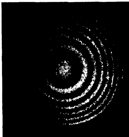
Figure 12.18. Moiré interferogram obtained when testing a spherical mirror ( \lambda_{eq} = 200\text{ }\mu\text{m} ).
