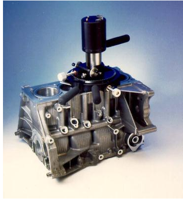
Insight 2000 measuring inside of engine bore
