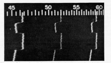
Fig. 7.79. Fringes of equal chromatic order given by a section of a diamond crystal surface. The scale is of wavelength in hundreds of Ångstroms. (After S. TOLANSKY and W. L. WILCOCK, Proc. Roy. Soc., A, 191 (1947), 192.)
