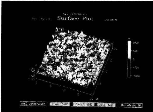
Figure 17. A 20x20  $\mu\text{m}$  image taken on an ABS with the SPM.
