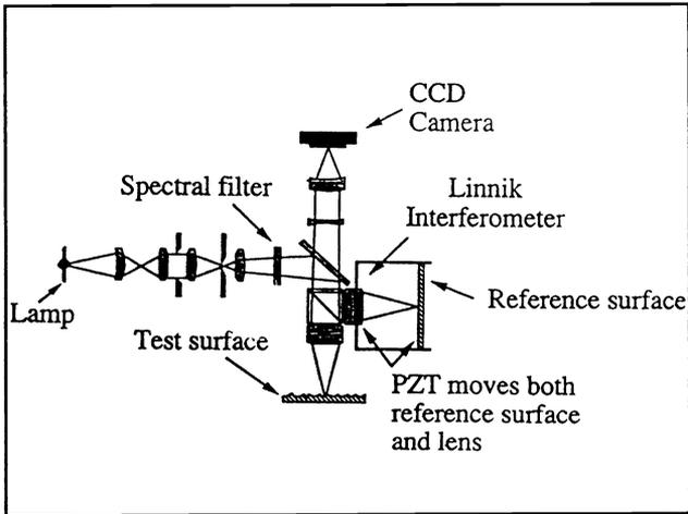
Figure 1. Schematic representation of an optical profiler.
