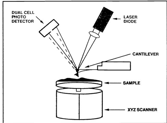
Figure 2. Schematic representation of a scanning force microscope.
