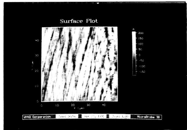
Figure 4. A  $50 \times 50 \mu\text{m}$  image taken on a magnetic disk with the SPM.
