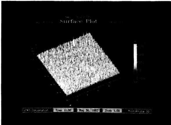
Figure 25. A 10x10  $\mu\text{m}$  image taken on a thin polycrystalline crystalline silicon film on silicon with the SPM.
