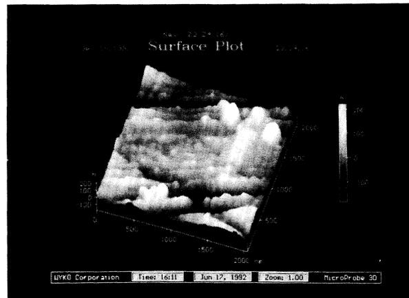
Figure 18. A 2x2  $\mu\text{m}$  image taken on an ABS with the SPM.
