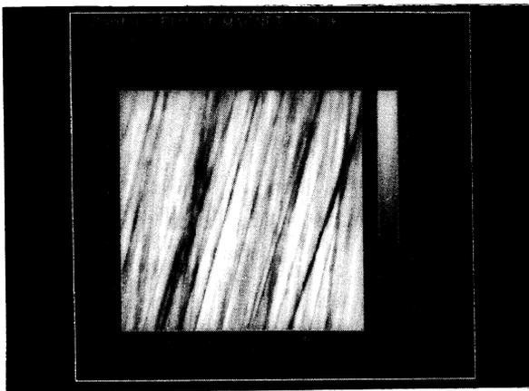
Figure 3. A  $50 \times 50 \mu\text{m}$  image taken on a magnetic disk with the optical profiler.
