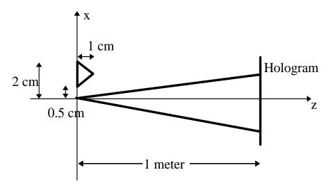
Note that the longitudinal magnification goes as the square of the lateral magnification.
