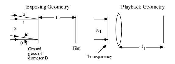
Two identical speckle patterns are recorded separated a distance =  $f \theta$ .
