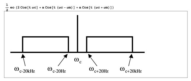
The bandwidth is 40 kHz. If the signal can be filtered, one of the sidebands and the carrier can be suppressed and the signal can be transmitted (single sideband - suppressed carrier) in a bandwidth of 19,980 Hz.
