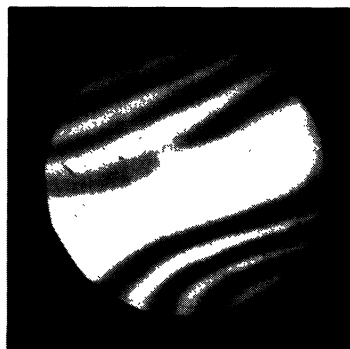
Fig. 7. Fringes given by a PDI with a narrow annulus as source and diffracting aperture.
