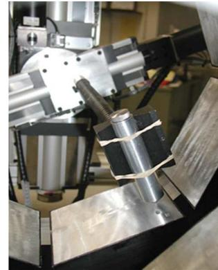
Fig. 4 *In situ* MDRF acquisition of a modular camera in FastSPECT II.
