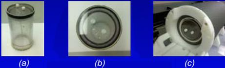
(a) Side view, (b) top view of the annular shell phantom and (c) with the phantom inside the SPECT system for system calibration
