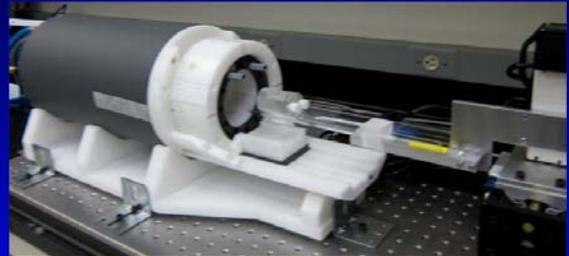
Experimental set up with the SPECT system set up with stepper motor and phantom on lab bench
