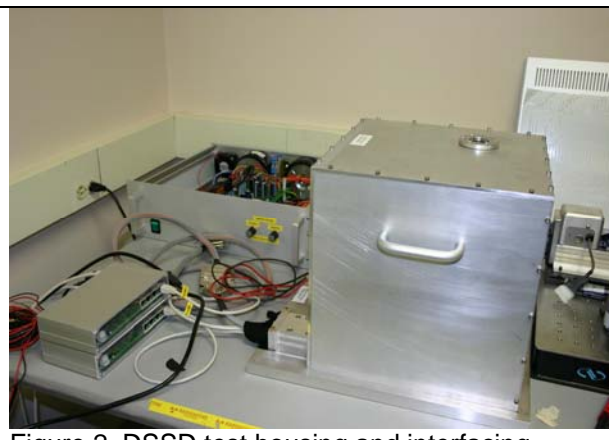
Figure 2. DSSD test housing and interfacing equipment
