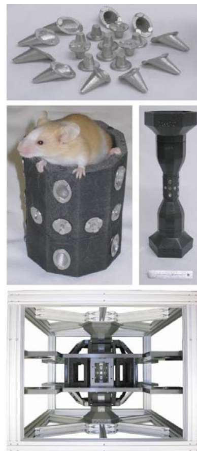
Figure 3. FastSPECT III imaging aperture fabricated using 3D rapid-prototyping printers and casting techniques. Top: platinum pinhole inserts made by lostwax casting methods; Middle: (left) cold-cast tungsten composite aperture with pinhole inserts; (right) complete imaging aperture; Bottom: imaging aperture installed in FastSPECT III.
