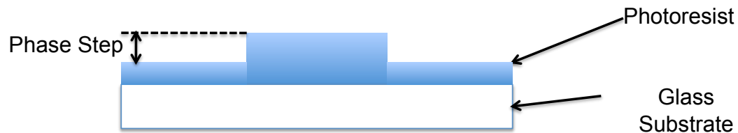
Figure 5.7: A cross-sectional view of a printed CGH. The height of the photoresist layer will produce the desired phase shifts in order for the CGH to reconstruct the image.
