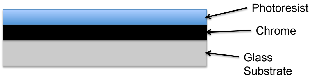
Figure 5.9: The binary mask slides are multilayered samples. The glass substrate is coated with a chrome layer and the chrome layer is coated with a layer of photoresist.
