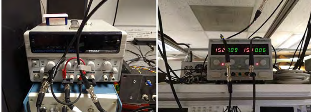
Figure 6.4: Commercial DC power supplies providing the \pm 15 V needed to power the 32 channel analog voltage output board from the computer. These power supplies output the necessary current to keep the computer output control voltages from drooping throughout an experimental run.
