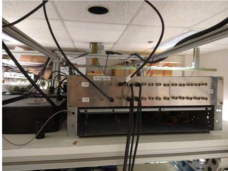
Figure 6.3: Home-built \pm 15 V and \pm 5 V power supply relegated to low current uses only.
