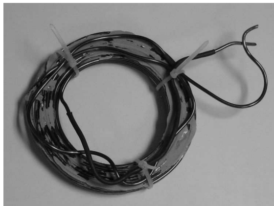
Figure 3.3: Photograph of a single magnet coil. The coil has an inner diameter of 6.5 cm.
