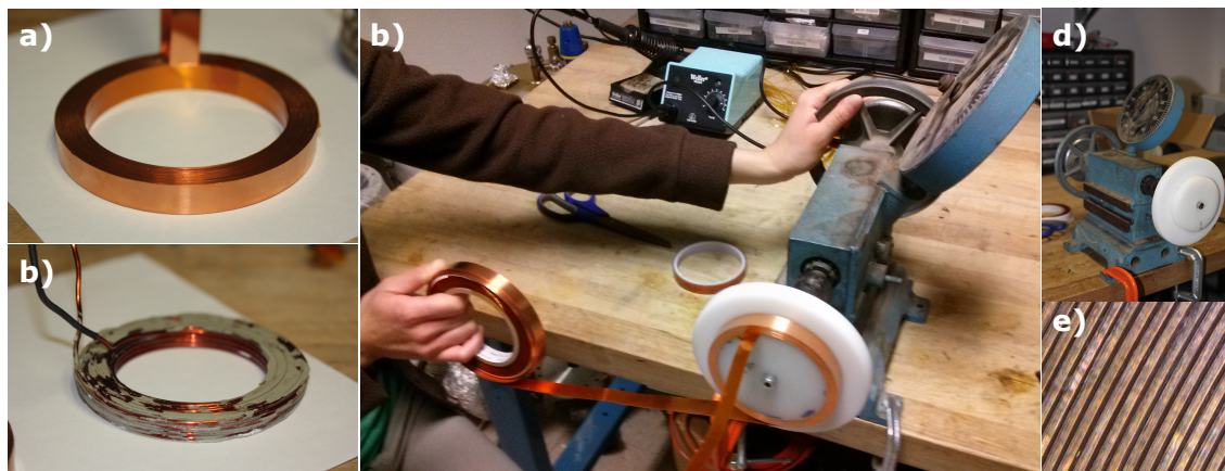
Figure 4.3: Overview of the transfer coil winding process. The image in d) shows the coil winding machine and the jig we use to wind the large transfer coils. c) A photo taken during winding process. Coil winding can be accomplished by one person; an extra set of hands makes the coil winding process very simple. a) and b) Show the difference between the transfer coils in BEC 1 (b) and BEC 2 (a). Coils wound with the thick copper tape are much more uniform and are easier to wind. e) Shows a close up view of one of the transfer coils and demonstrates the uniformity and regularity of the copper tape-style coils. The uniformity in winding leads to more efficient heat dissipation.
