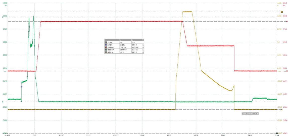
Figure B.5: Picoscope trace of the total transfer coil current (green), the measured current through the BEC quadrupole coils (red) and the photodiode signal proportional to the 1064-nm laser power (yellow) without RF on during the run.
