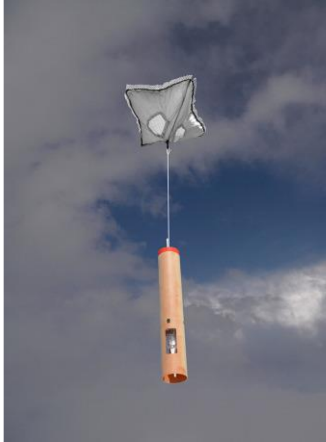
Figure 9: Picture of NCAR AVAPS NRD41 dropsonde when launched from aircraft (Vömel and Dunion, 2023).
