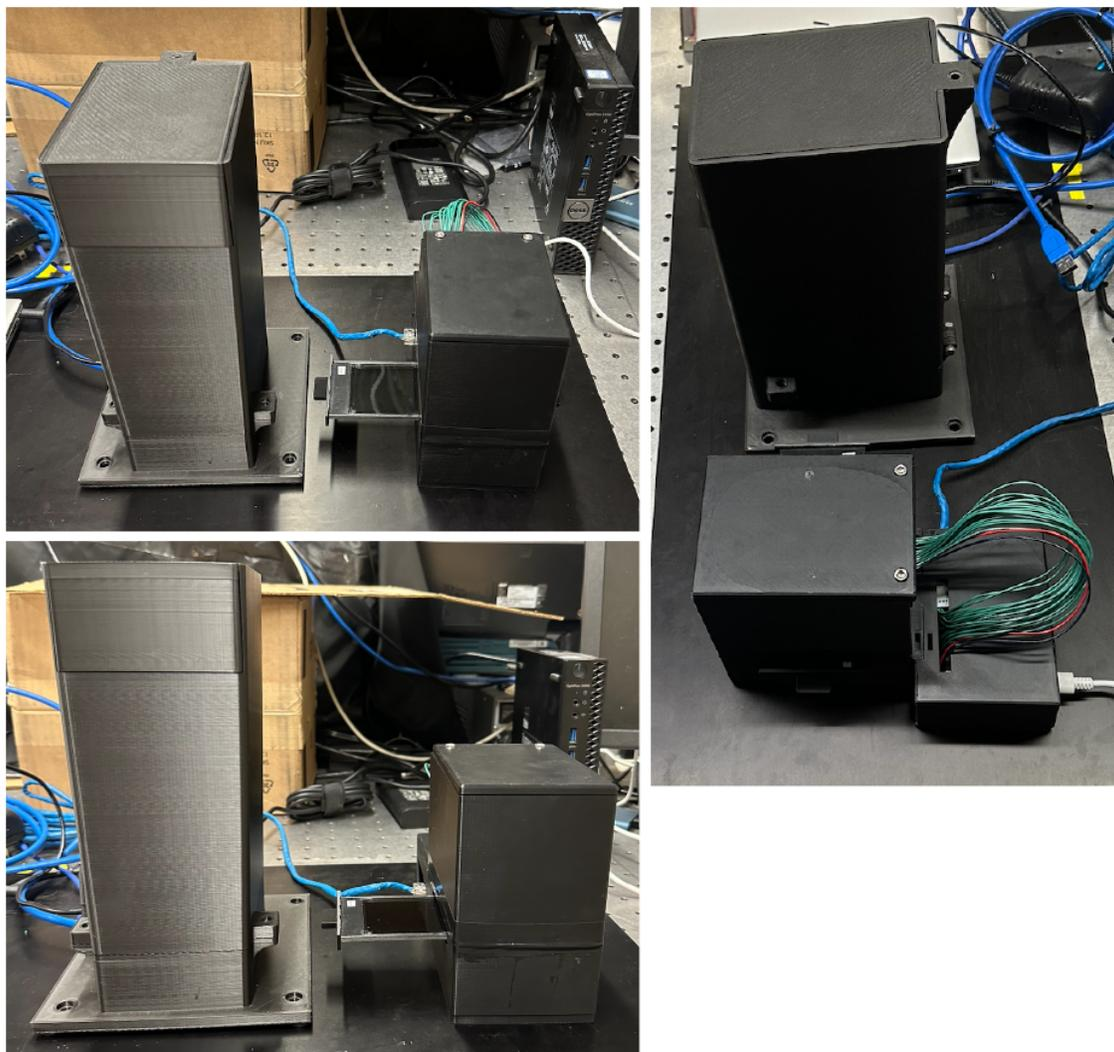
**Figure 5.5:** Comparison of two LFHM devices. Both LFHM devices used in this dissertation are shown side-by-side. On the left side of the images is the QLAB sensor used in SARS-CoV-2 quantification in Chapter 3, and on the right is the new P-LFHM sensor, which stands half as tall with a similar footprint as the QLAB sensor.
