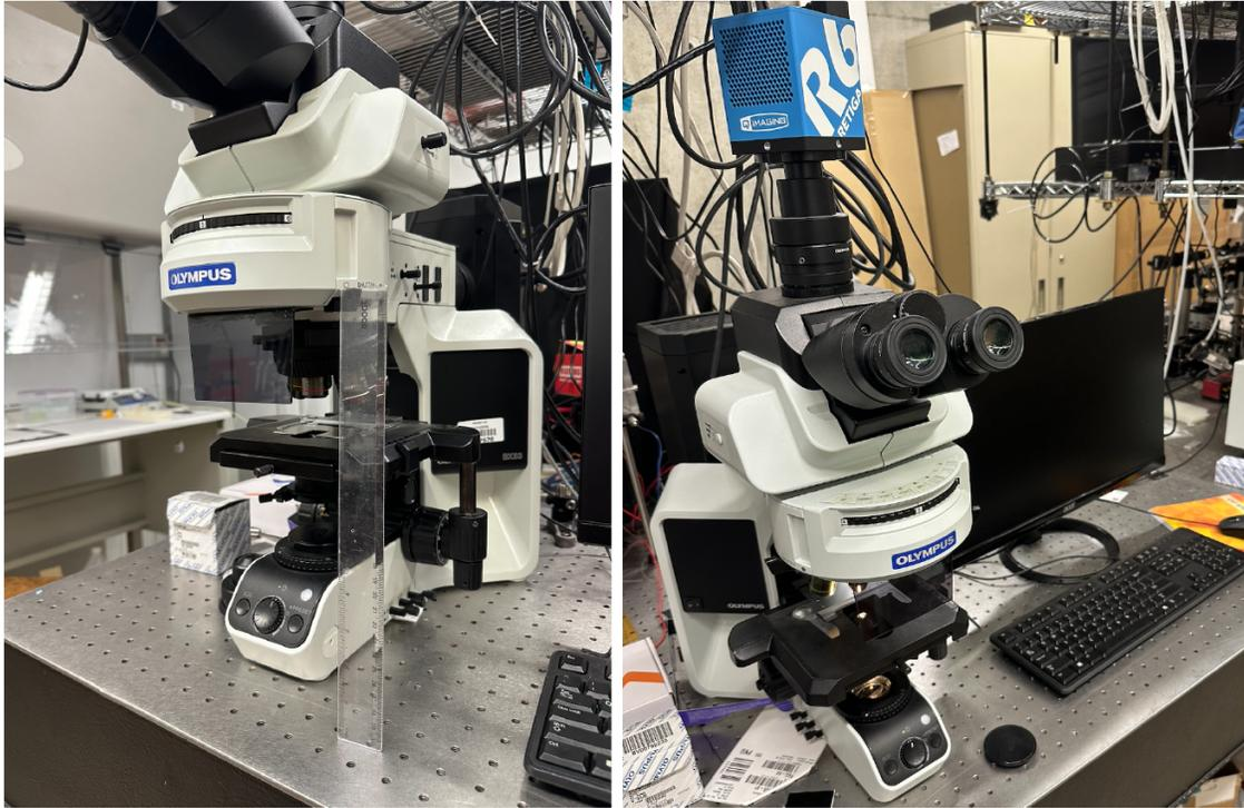
**Figure 1.7:** Brightfield microscope. This is the Olympus BX53 microscope. It acts as a bright-field, darkfield, and fluorescence imaging microscope. Of note are its large size which makes this microscope non-portable, and its cost which is \$6,300.
