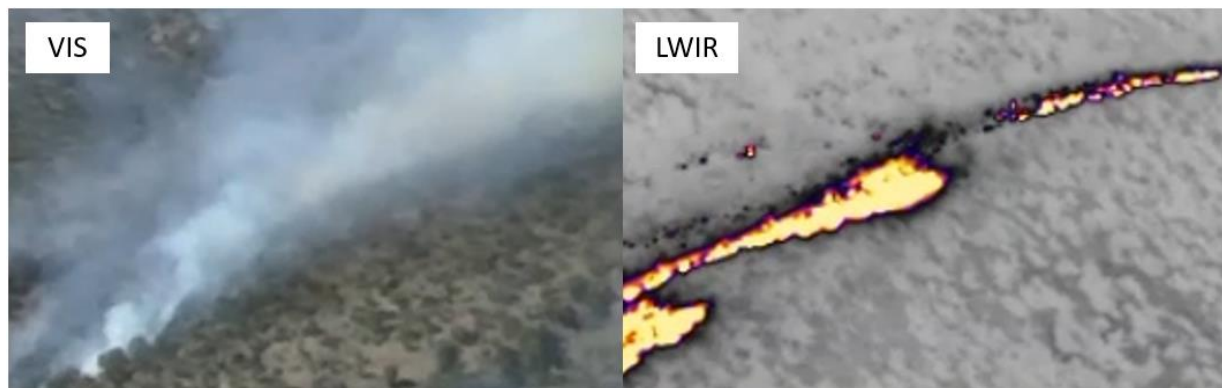
Figure 6.1: Overlapping VIS and LWIR aerial imagery demonstrating the current imagery obtained by the Zenmuse XT2 system. This imagery was provided by a Southwest Region Forestry service drone pilot. (LWIR imagery is white cold and black hot with an unknown color threshold)
