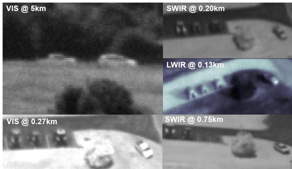
Figure 5.8: Frames from different test sequences from the data collection that imaged the truck, van, and tractor in the 3 different bands being studied.
