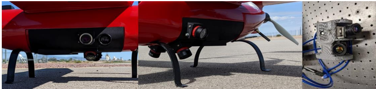
Figure 5.4: WAC systems in their custom housings attached to an Event38 E400 VTOL drone. The 6-Camera visible is on the left, the 4-camera SWIR is in the center and the 4-camera LWIR is on the right.
