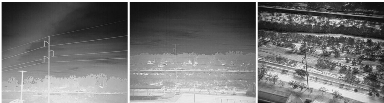
Figure 4.1. Power Lines in the LWIR. Figure 4.1a (left) shows the wires against a cold sky where the ground reflection makes the wires bright. Figure 4.1b (middle) shows where the wire radiance matches the sky path radiance (i.e., no contrast). Figure 4.1c (right) shows a look down where the wires are dark reflecting cold sky against a warmer ground background.
