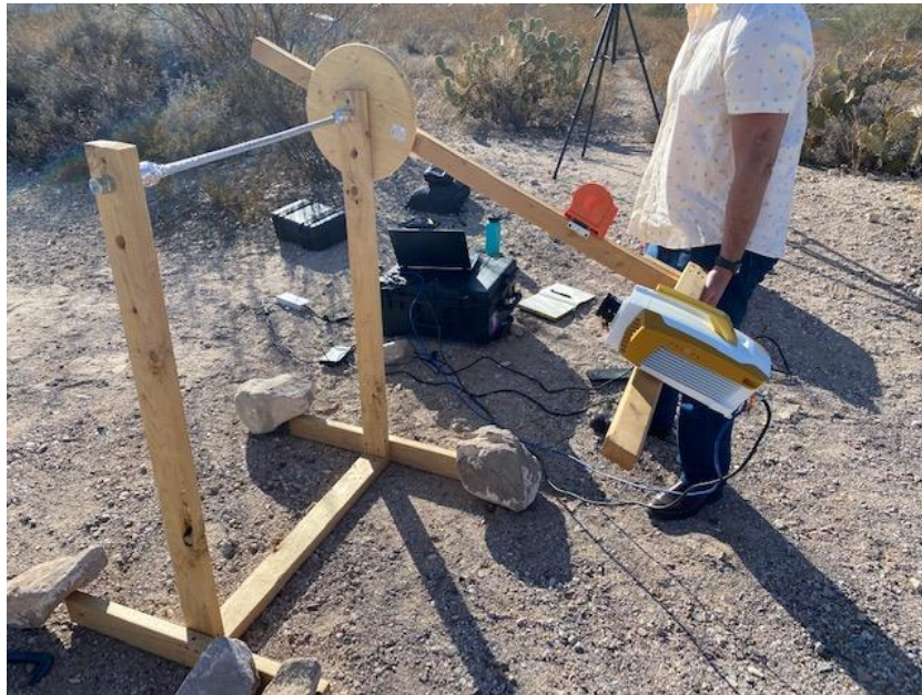
Figure 4.4: Apparatus which holds the either the LWIR sensor or MWIR sensor (pictured) which contains the wire in the middle of the rotational axis, an arm holding a sensor at a constant distance, an inclinometer on the arm and a large disc to clamp the arm in place.
