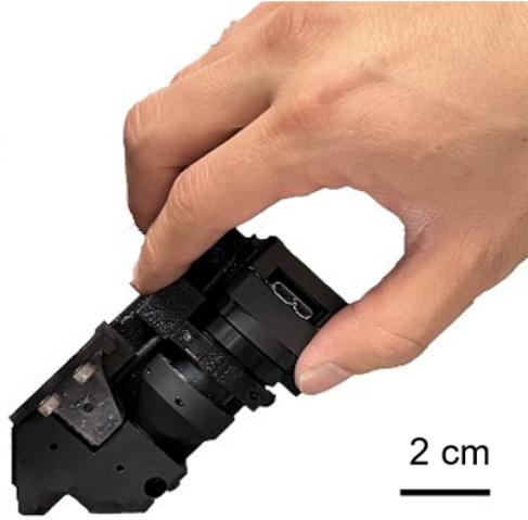
**Figure 5.4:** Photo of the sLSM probe.
