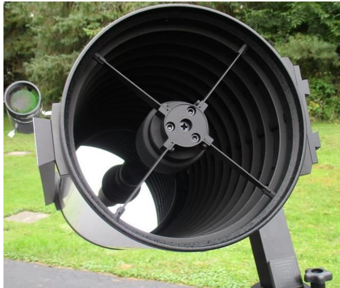
Figure 5: Cassegrain obscuration, courtesy of L. Carlino's article "GSO 8-Inch True Cassegrain"
