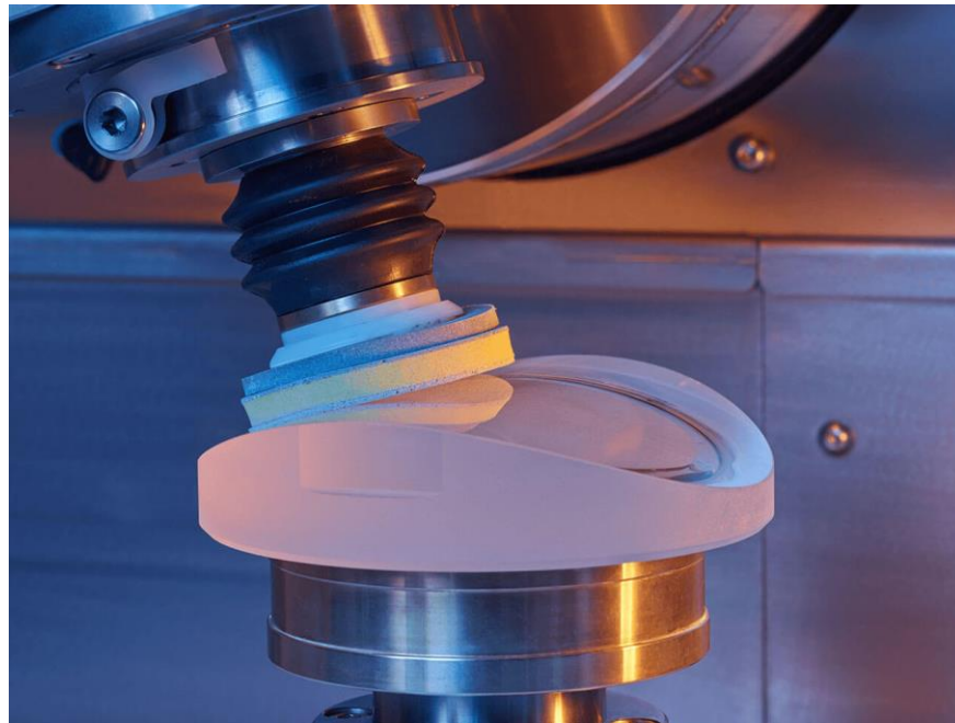
Figure 11: CNC optical polishing machine, Satisloh
