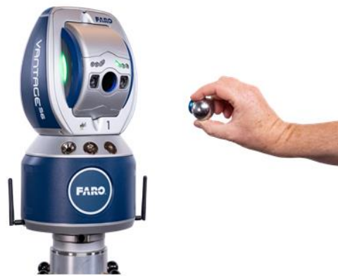
Figure 13: FARO laser tracker with an SMR
