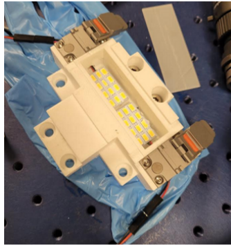
Figure 5.2: Workpiece holder used for grating fabrication.
