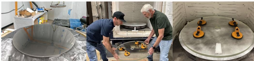
Figure 2.18: Precision polished steel mold (left), lifting the 32" BOROFLOAT® mirror into the oven (center), and the slumped glass blank on the mold surface in the oven (right).
