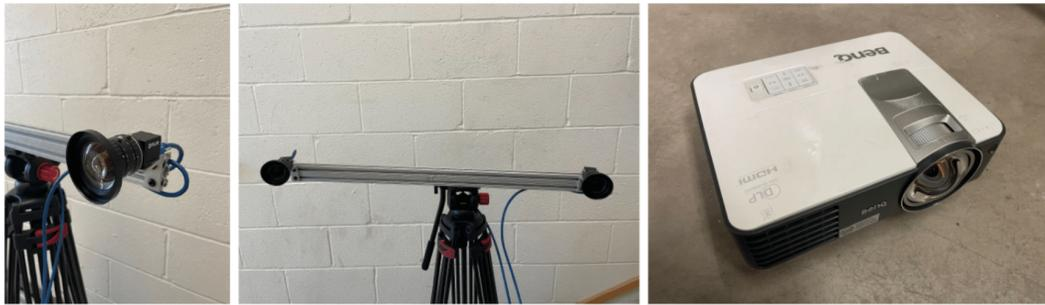
Figure 4.3: Left, one of the two FLIR Blackfly USB3 cameras with 8 mm focal length lens. Center, both cameras mounted to 8020 aluminum extrusion, mounted to a tripod. Right, BenQ 1080P short-throw projector used in this experiment.
