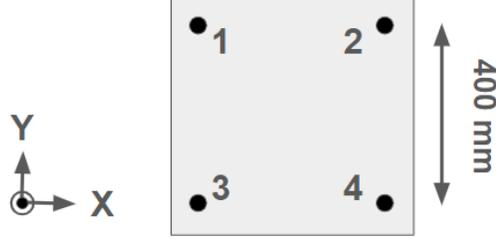
**Fig. 4** Coordinate system and actuator layout for each panel. Once tip, tilt, and piston values are extracted, they need to be converted to actual numbers of rotations on the actuators.
