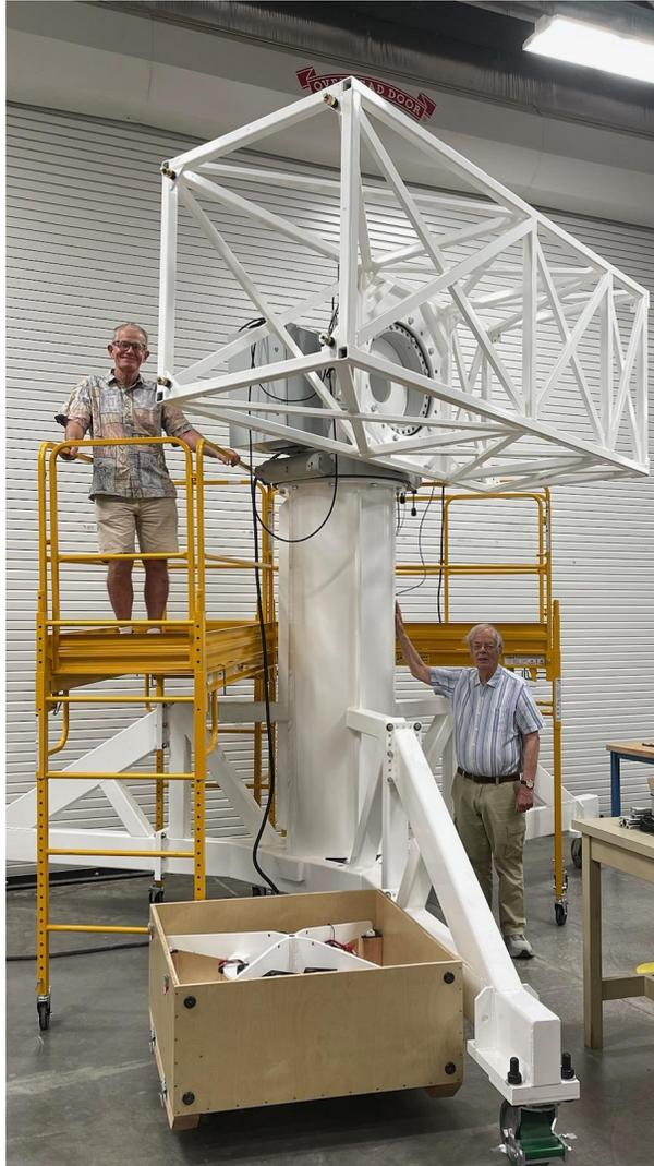
Figure 2.23: The final painted frame for the single unit telescope. It uses the same azimuth and elevation drives and the same pier that the 20-unit telescope will use.
