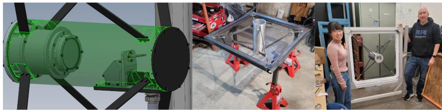
Figure 2.22: CAD drawing of the PFC barrel (left), the barrel attached to its mounting structure (center), and the final PFC barrel populated with the lens assembly with graduate student Sonja Choi and Dr. Andrew Monson. (right)
