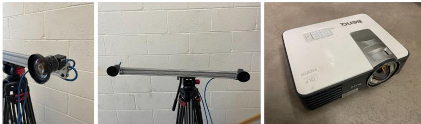
**Fig. 5** Left, one of the two FLIR Blackfly USB3 cameras with 8 mm focal length lens. Center, both cameras mounted to 8020 aluminum extrusion, mounted to a tripod. Right, BenQ 1080P short-throw projector used in this experiment.
