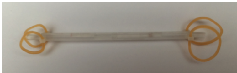
Figure 5.2: Vessel phantom 3 mm in diameter. There are four elastic bands (yellow) for hanging inside the MOCOMO phantom.
