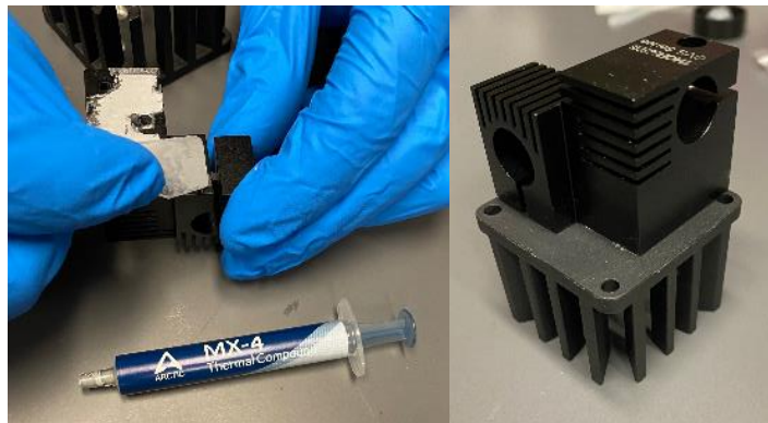
Figure 7: Attaching the galvo holder to the heat sink.
