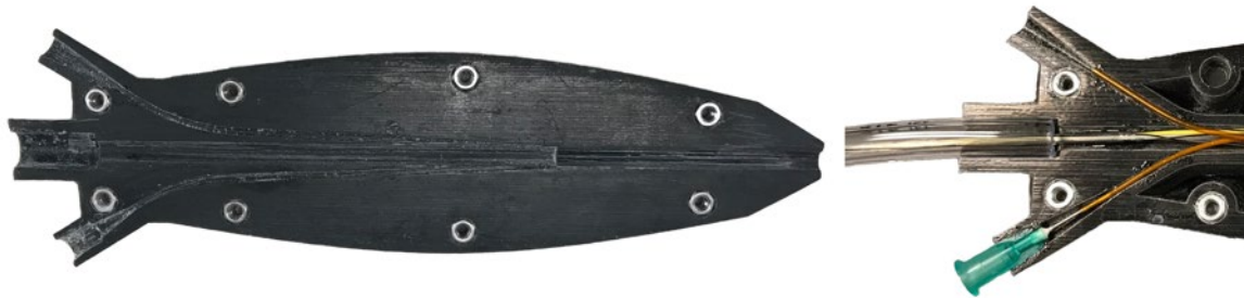
Figure 9, (Left) Open handle showing the internal channels guiding the different components. (Right) Handle with components installed.
