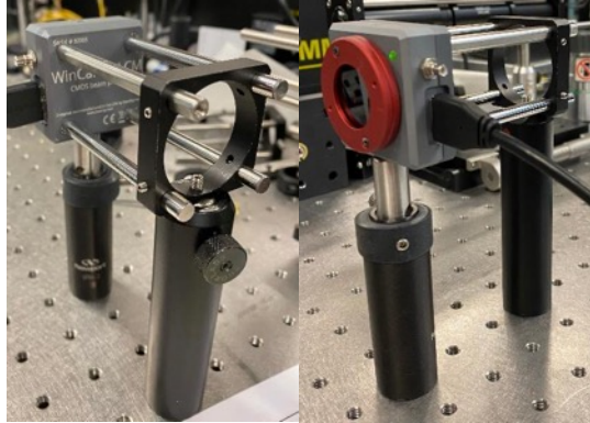
Figure 9: Setting up the alignment tool that will keep the camera from tilting about the y-axis.
