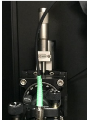
Reference arm translation stage used to modify and adjust the OPD.
