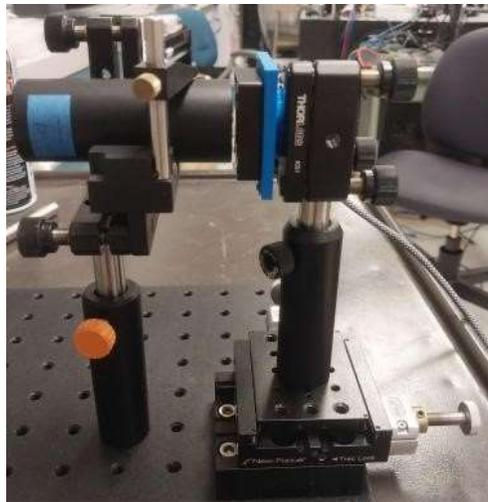
*Figure 11: Setup used for slanted edge MTF testing of the objectives*
