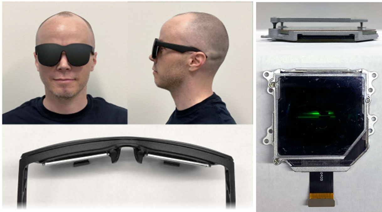
Figure 28: (Left) Sunglasses prototype. The driving electronics and light sources are mounted externally. (Right) Display module for this prototype. Consists of a backlight, display panel, and eyepiece. The total thickness of the module is 8.9mm [Maimone, 11]
