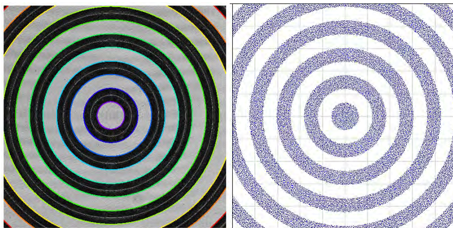
FIGURE 5.29 The final detected rings color coated in order of size and overlaid on top of the modulation data (Left), and an image generated by the Zemax model after optimization (Right).
