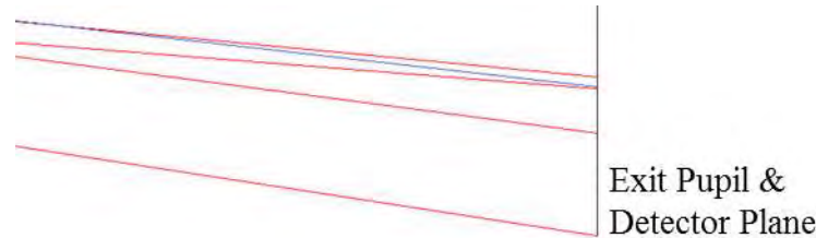
FIGURE 4.28 The spread of the possible test rays at the edge of the exit pupil which all originated from the same point on the edge of the intermediate pupil. In a given interferogram there is only one test ray present for any point in the pupil. Therefore the size of the test wavefront at the exit pupil depends on the slope of the test ray in the intermediate pupil and the transverse ray error of the imaging lens.
