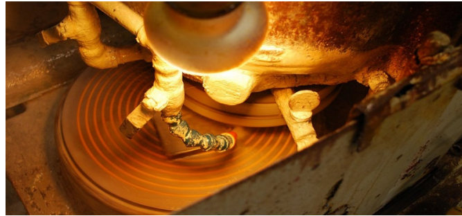
Figure 25: Initial Shaping Process of flat to remove subsurface damage using Blanchard Mill with 180 Grit Wheel.
