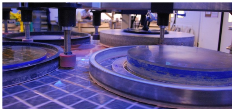
Figure 27: Substrate on Polishing Lap for final angular correction and surface figure production
