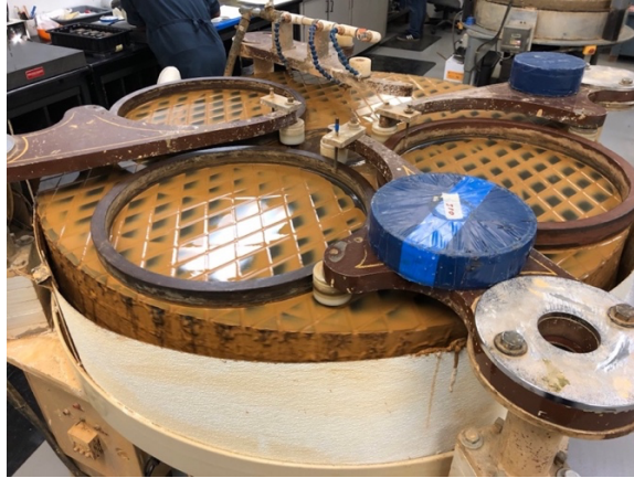
Figure 26: Grinding Laps being prepared to grind substrate with 15 Micron Grit
