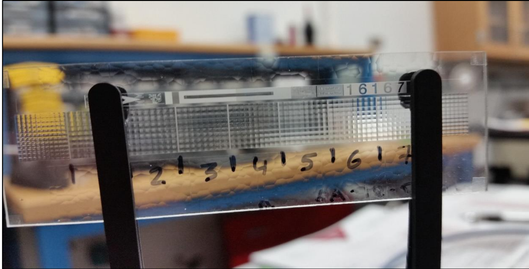
Figure 3.3: Image of lenslet arrays from RPC Photonics. Each 10×10 array offers a different option for lenslet focal length.
