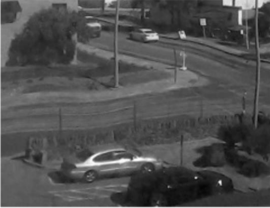
Figure 2.4: Example of local distortions due to imaging through anisoplanatic turbulence. This is most evident in the light pole on the right side of the picture as well as in the curb lines in the central and upper right portions of the image. Image courtesy of Michael Hart.
