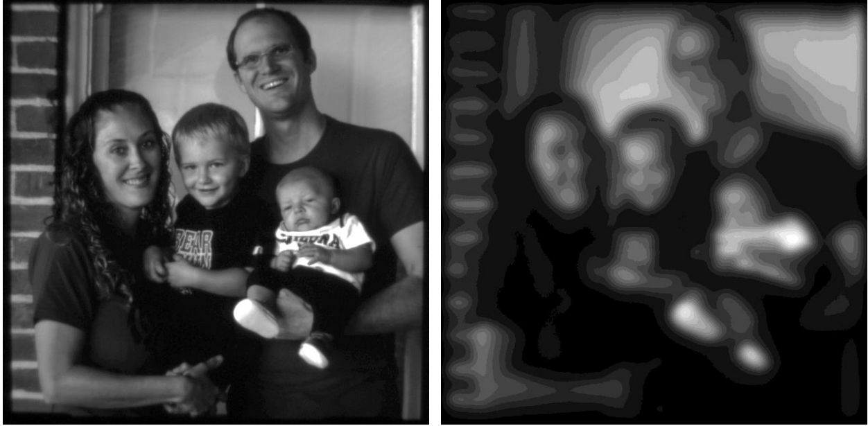
Figure 3.15: An image of the author's family as seen by the science camera. The image on the left shows the scene prior to disturbance by atmospheric aberration. The image on the right is compiled from 100 frames taken through dynamic phase screens. There is also some residual defocus included in the right image due to the addition of the optically thick phase plates.
