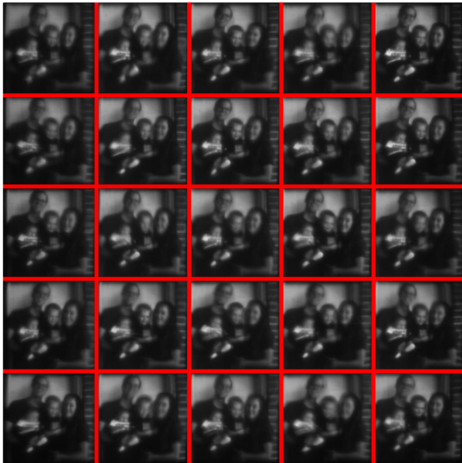
Figure 3.17: Example of a frame from the WFS lenslet arm. Each sub-image is separated and analyzed independently.
