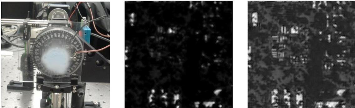
**Fig. 21.** USAF target with Optispray diffusing material on it to emulate diffusion (left), sample of LR image taken with  $NA_{meas} = 0.037$  (center), and the resulted FP reconstruction of  $NA_{synth} = 0.1$  (right).
