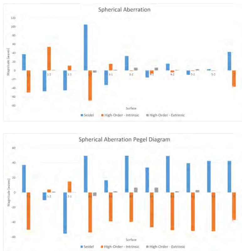
**Fig. 2.7** Surface contributions to the symmetry of spherical aberration and associated Pegel diagram for a flat field design (benchmark lens) and a representative lens imaging on a curved sensor (evaluation lens).
