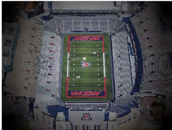
**Fig. 3.5** Stadium at the University of Arizona simulated through an early wide-angle lens (US 2031792). Sharp decrease in illumination toward the corners of the image limits the field-of-view of the objective.
