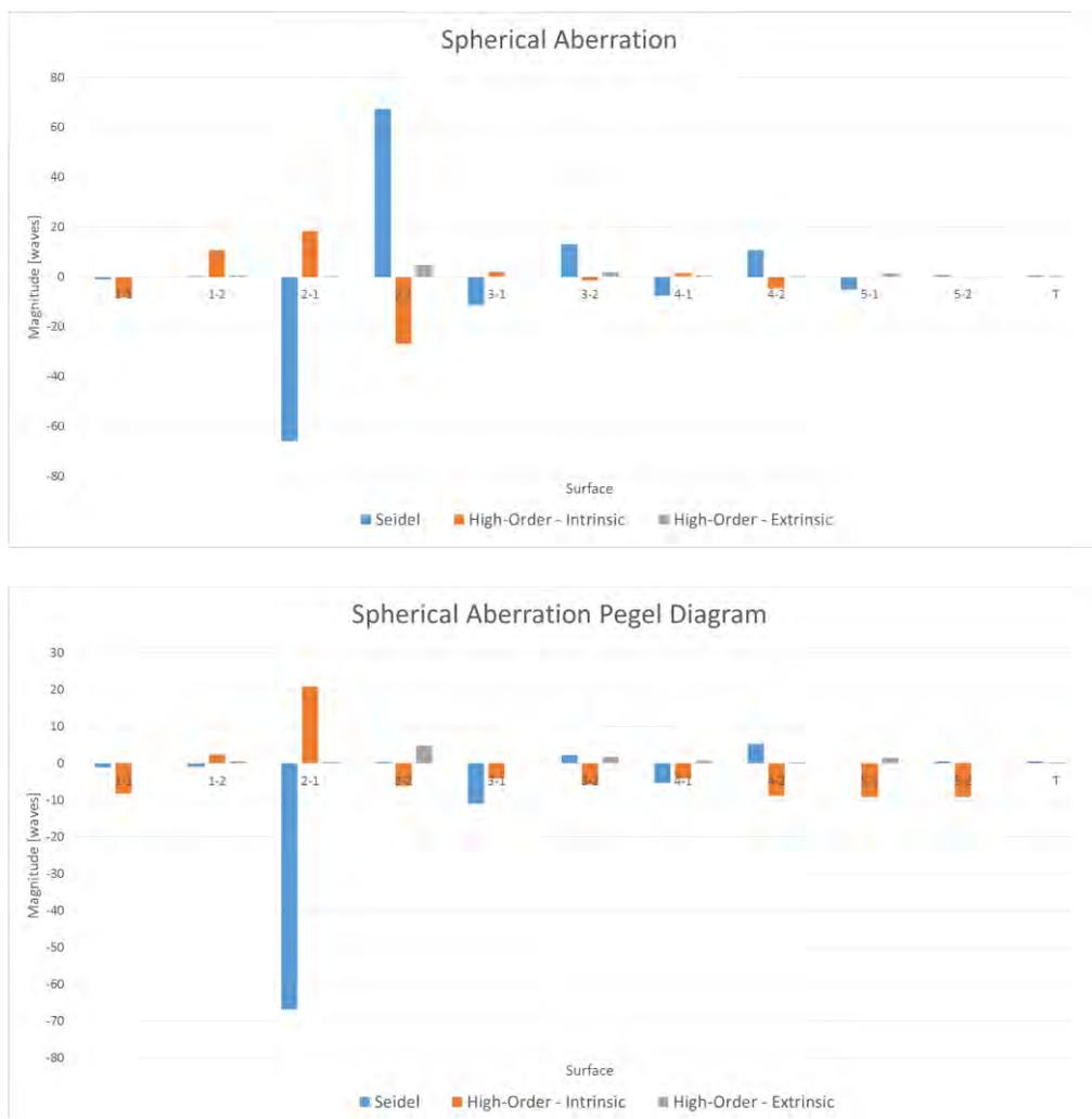
**Fig. 2.6** Surface contributions to the symmetry of spherical aberration and associated Pegel diagram for a flat field design (benchmark lens).
