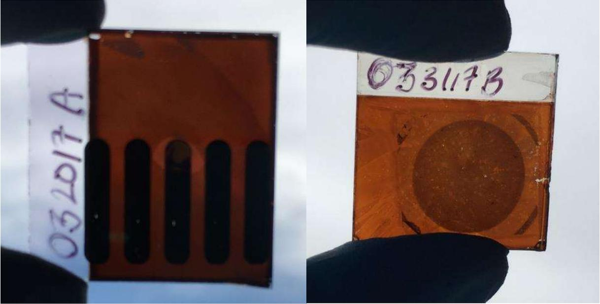
Figure 6.10. (left) Completed perovskite solar cell with evaporated back electrode. (left) Completed perovskite solar cell with CuNW back electrode.
