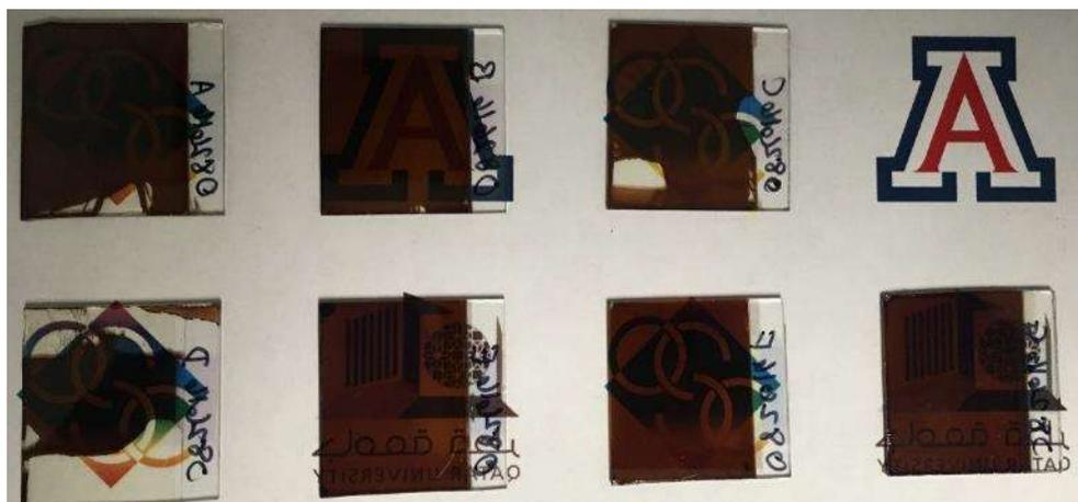
Figure 5.9. Photograph of high-temperature-ETL perovskite cells showing the variance during spin coating based on precursor used, and ETL surface roughness.
