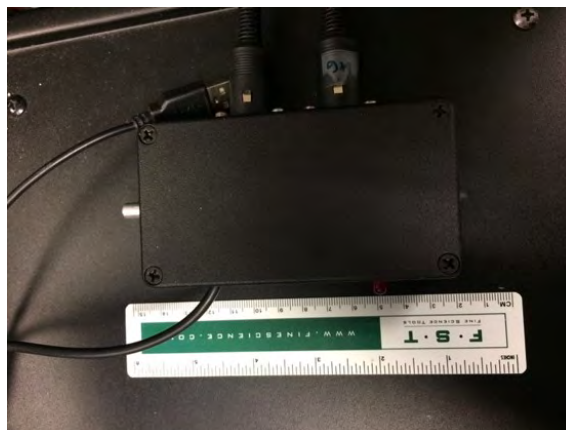
Figure 2.22: Box for controlling the gain of PMTs. A potentiometer controls the gain voltage through a divider circuit. A LED indicates the on and off status
