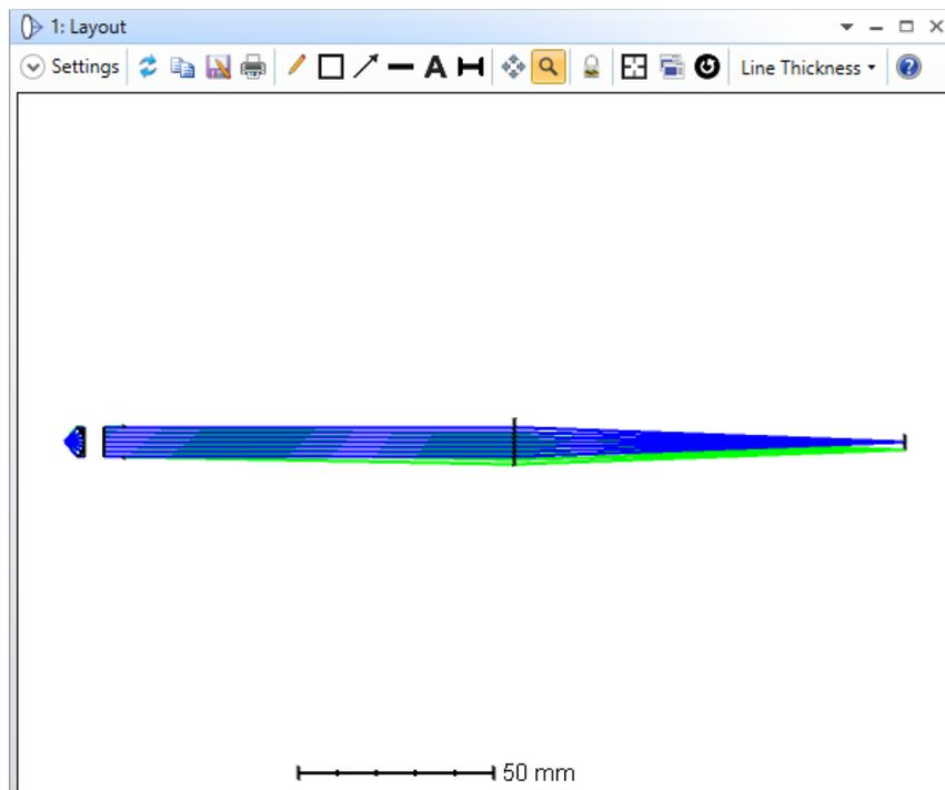
Figure 3.10 Lay out of thin lens with principal plane model.
