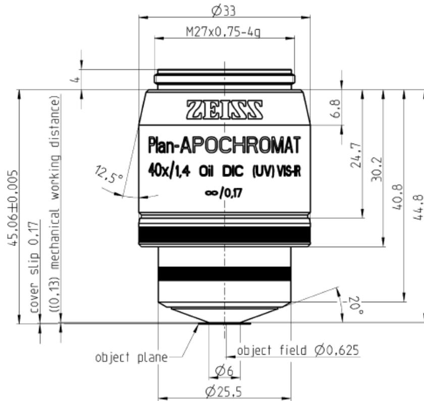
Figure 2.13 Mechanical dimensions for a Zeiss plan-apochromat objective.
