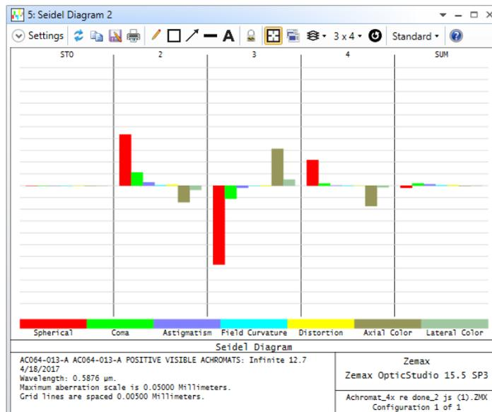
Figure 4.13 Seidel diagram of the achromat (c).
