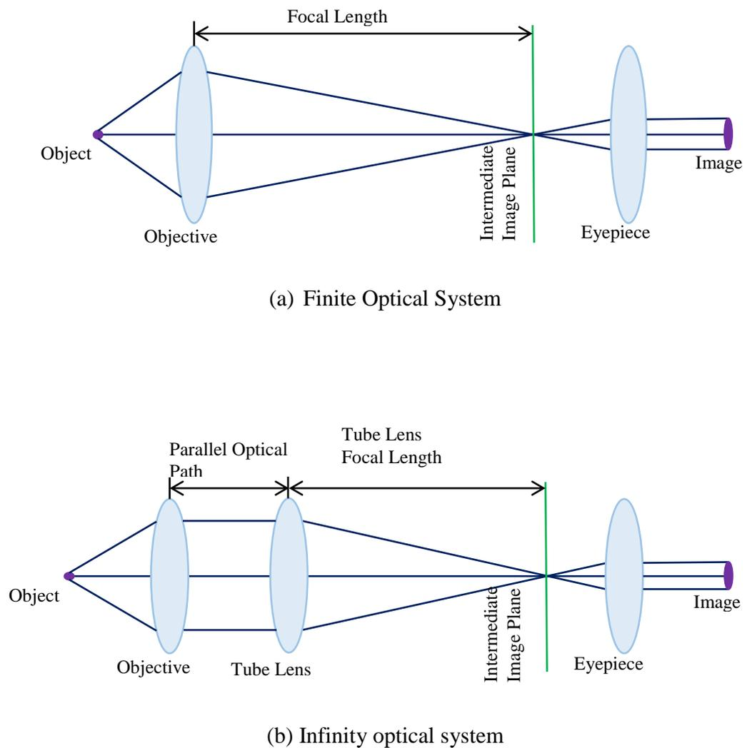
Figure 2.8 Finite & infinity microscope optical system.
