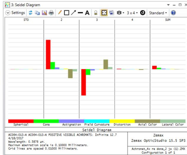
Figure 4.8 Seidel diagram of the achromat (b).
