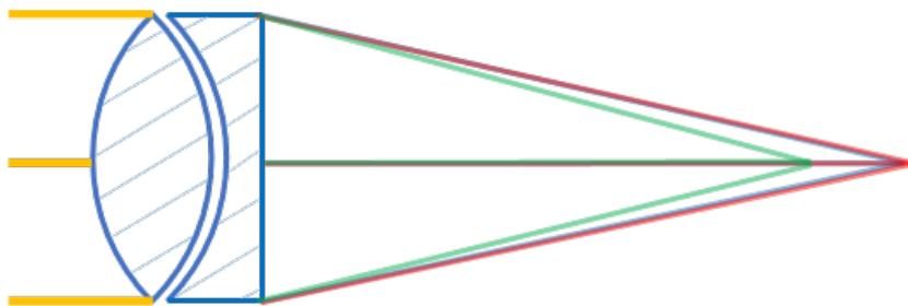
Figure 2.11 Chromatic aberration correction of an achromat.
