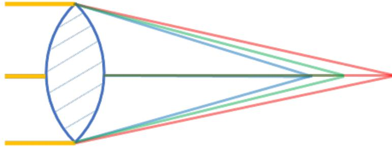
Figure 2.10 Chromatic aberration of a single lens.
