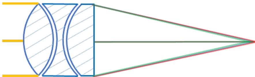
Figure 2.12 Chromatic aberration correction of an apochromatic objective.
