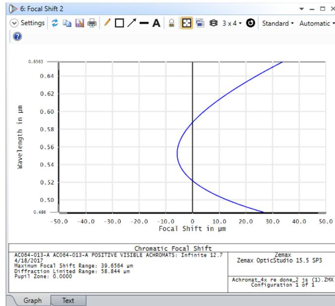
Figure 4.12 Focal shift of the achromat (c).
