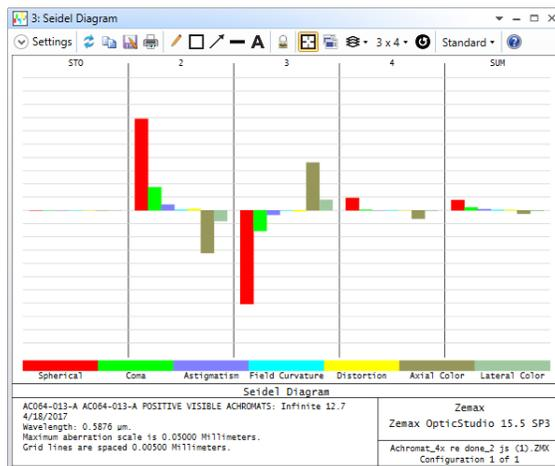
Figure 4.5 Seidel diagram of the achromat (a).
