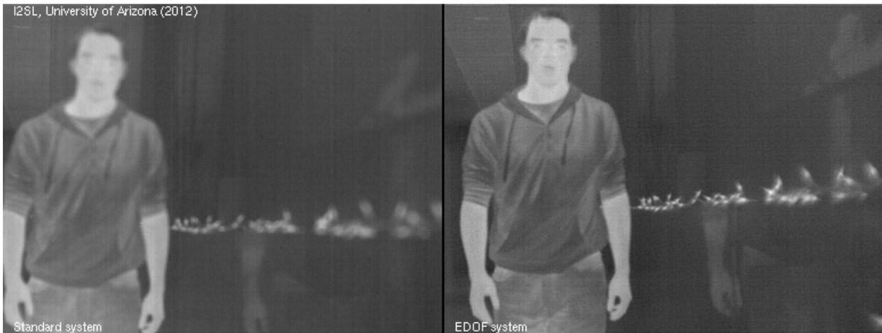
Figure 2.21: Side by side comparison of a natural scene. On the left is the image produced by the standard system (a FLIR camera) and on the right, by the EDoF system (an identical FLIR camera, with the phase mask mounted and after the digital reconstruction of the stream). For both side, the cameras are focused at 25.0m and the person is standing at approximately 4.0m. Note that the closest light bulbs on the right side are at a distance of 2.0m.
