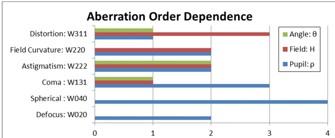
**Figure 9: Aberrations that effect scan lens design, and their azimuthal angle, field height, and Pupil height dependence. (11)**
