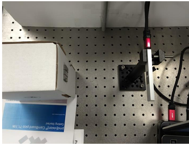
Fig. 14. Example setup with ToF camera viewing gauge blocks.
