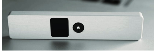
Fig. 13. Photo of time-of-flight camera unit. Illumination port on left; detection lens on right.
