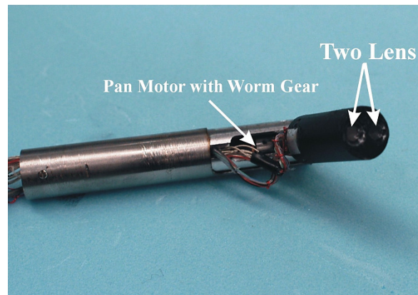
Fig. 6. Example of binocular stereoendoscope, from "Insertable stereoscopic 3D surgical imaging device with pan and tilt" by Hu et al. [4] Although pan-tilt capability may be a desirable workaround for the field-of-view limitations, it involves significant tradeoffs in mechanical complexity and is not frequently implemented in commercial endoscopes. The tube diameter is 15mm, which is the practical limit imposed by the surgical tools used to create and maintain the incision.
