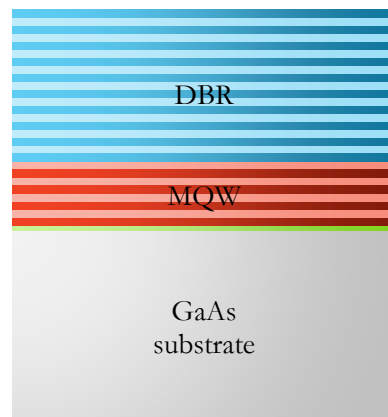
Figure 2.2 “Bottom emitter” design of VECSEL structure.
