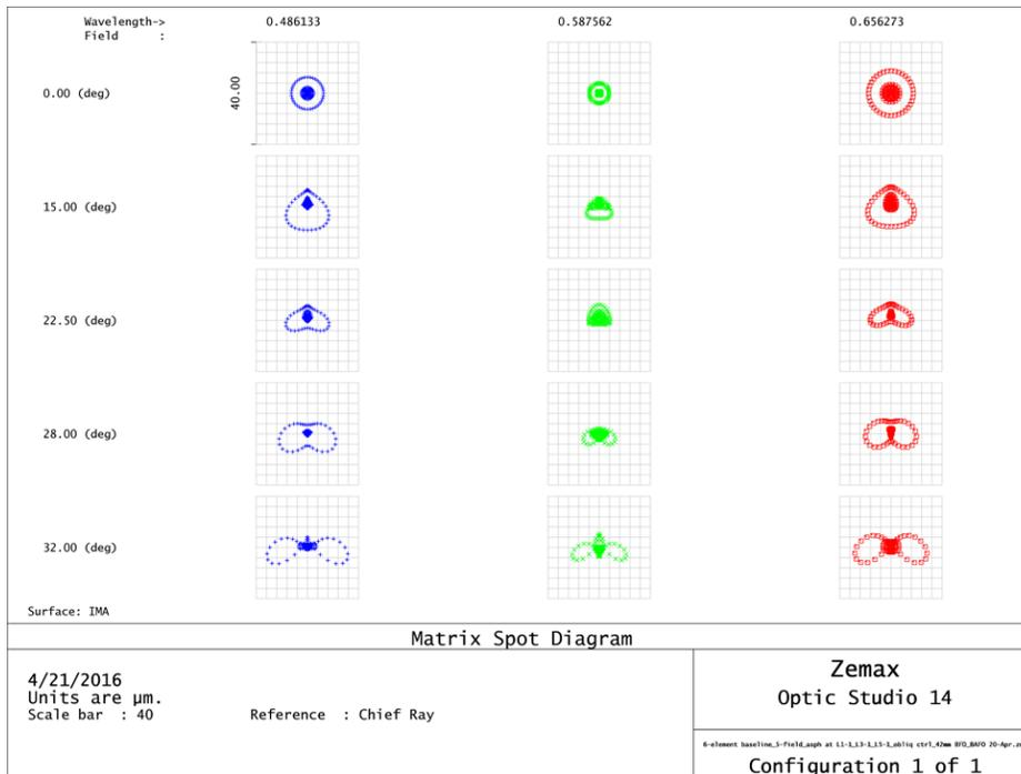
Figure 19 – Matrix of geometric spot diagrams for the baseline retrofocus lens across wavelengths for all fields.
