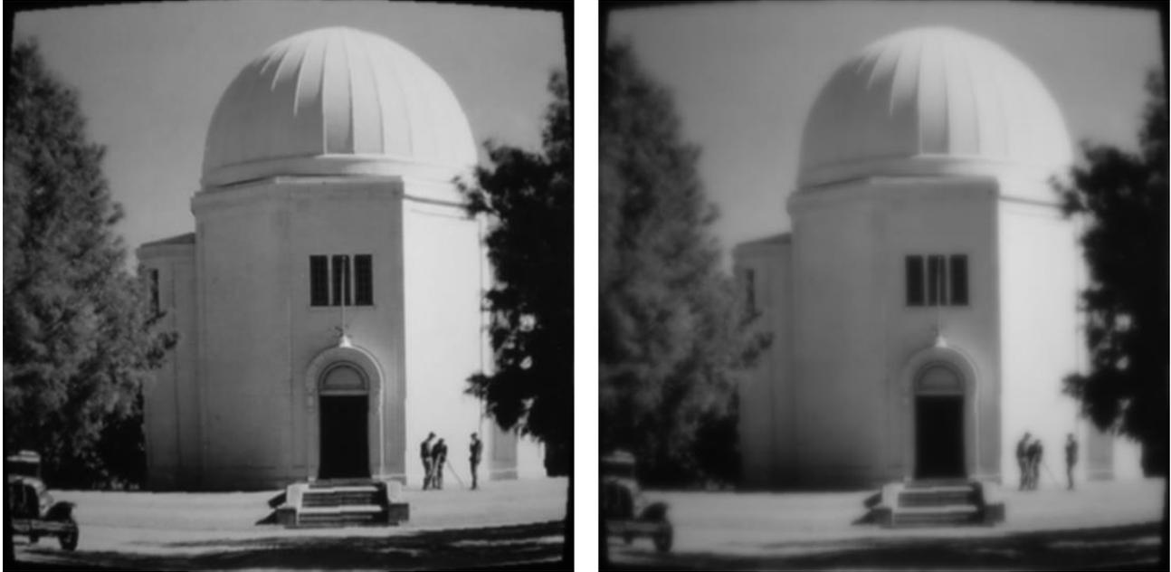
Figure 48 – Image distorted and blurred by baseline lens (left) and invariant lens (right)
